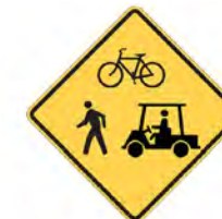
Custom combined pedestrian, golf cart, and pedestrian warning sign based on standard MUTCD warning sign
